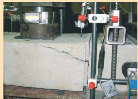
Typical "pop-out" failure of tested dowel systems
